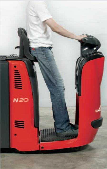
**Access and platform** Wide 390 mm entry on both sides and low 120 mm step-in height allow easy access to the truck. Absence of sharp corners and edges adds to operator safety and comfort.
