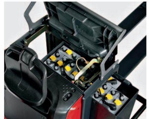
**Easy battery change** Optional side change (left or right) is available and includes a dedicated retainer system that locks the battery securely inside its compartment. Using the creep control buttons, the battery can quickly be lined up with the change stand and then raised by the initial lift for smooth changeout. With the five-point configuration, the active side stabilizers are blocked to maintain the truck in horizontal position when removing the battery.
