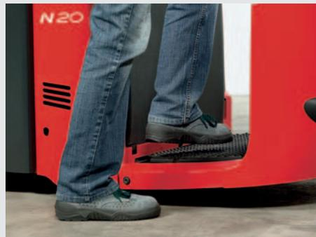
The full-suspension platform eliminates vibration. Its total area of 400 x 600 mm serves as a deadman zone and is covered with a soft, non-skid rubber mat providing highest standing comfort.
