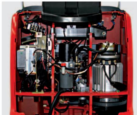
**Moisture- and dust-proof motor** AC drive technology incorporated in the new N20/24 does not require any maintenance. Rapid and convenient access to all internal components is provided by simply removing the front service panel.
