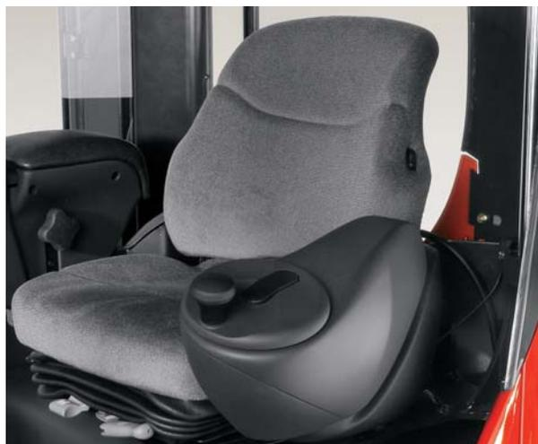
**Lift height preselector** is programmable for up to 99 shelf levels for safe, precise and economical load handling at any height.
