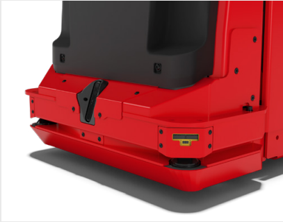
Safety laser scanner and 3D camera for environmental monitoring
